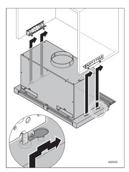
■ Fit the cooker hood into the wall unit from below, guiding it over the safety notch, as shown. Push it back until the spacer strip is flush with the wall.
